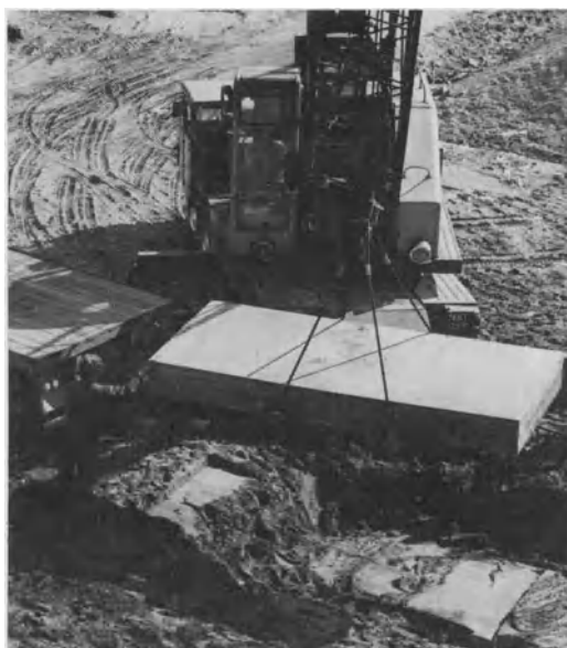
FIG. 5.6 Clad slab after firing.
