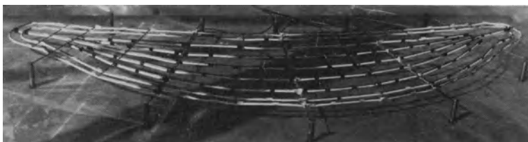
FIG. 9.6 Near-contact explosive charge positioned over dished pass partition plate forming blank.
