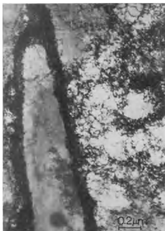
FIG. 3.28 Dislocation substructure generated by conventional deformation of shock-loaded nickel (25 GPa, 2 \mu s) in a tensile test. The elongated cells are associated with work softening.
