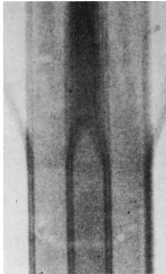
FIG. 10.6 X-ray flash pattern of an explosive compaction of Al-powder, exposure time 120 ns.
