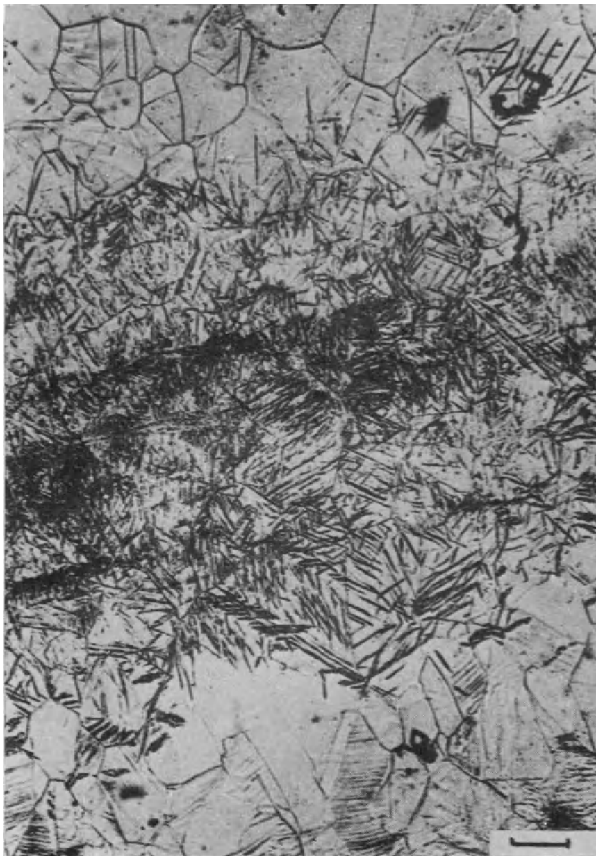
FIG. 2.25 Martensite generated by tensile hydrostatic stresses produced by a reflected pressure pulse in an iron-nickel alloy (from ref. 134). Bar = 100 \mu\text{m} .
