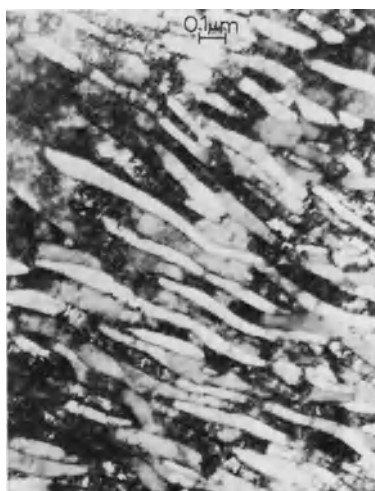
FIG. 3.15 High-pressure (120 GPa) sub-grain microstructure in 304 stainless steel resulting from shock-thermal effects (compare with twin-fault microstructures shown in Fig. 3.9).
