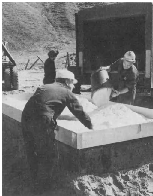
FIG. 5.5 Loading explosive on a stainless steel clad slab.
